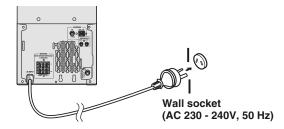
• Unplug the AC power lead from the wall socket if the unit will not be in use for a prolonged period of time.
